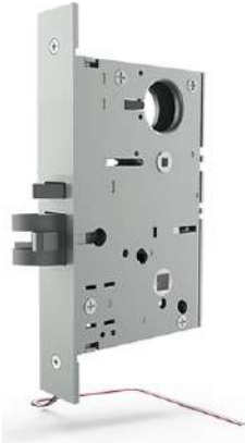
MT5907-SF (fail safe) MT5907-S (fail secure) Mortise lockset without deadbolt
